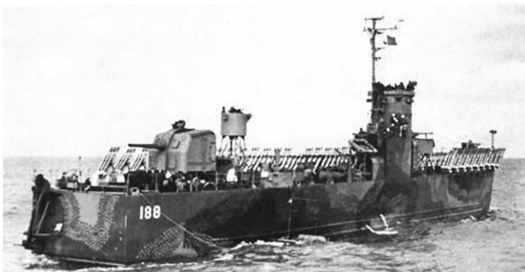
A photograph of a second generation LSM. These LSM's were completed as LSM's and then modified to take multiple racks of 5" rockets which covered the entire cargo deck. They were very effective in providing a creeping barrage for assaulting troops on a beachhead. Some 40 were converted. All were fitted with a 5" gun aft.
